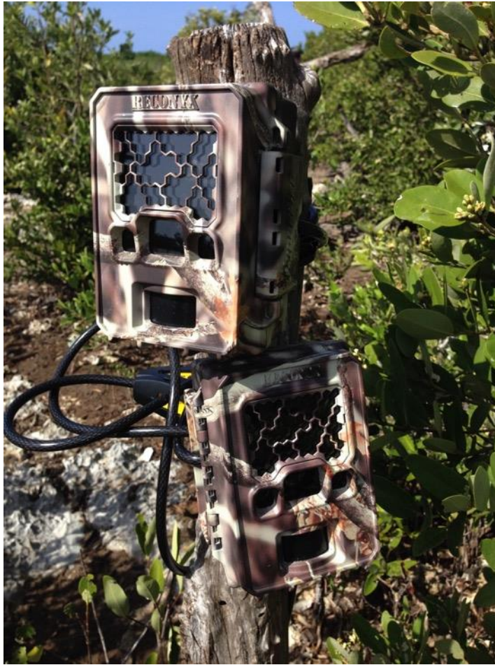
Fig. 5.1 Reconyx cameras deployed at the Booby Pond Nature Reserve (June 2016 onwards), to monitor red-footed booby nests.
